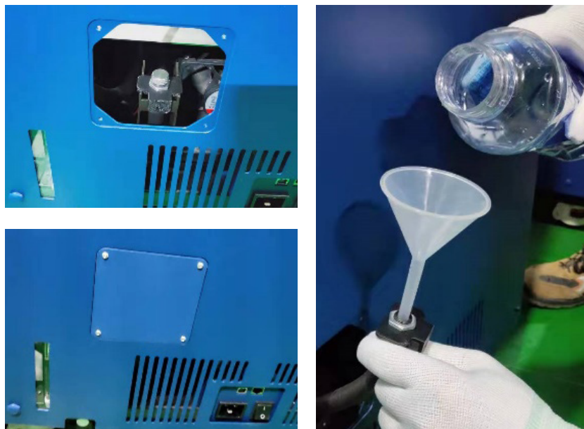
Figure 2.8 Position of charging inlet and method to charge
