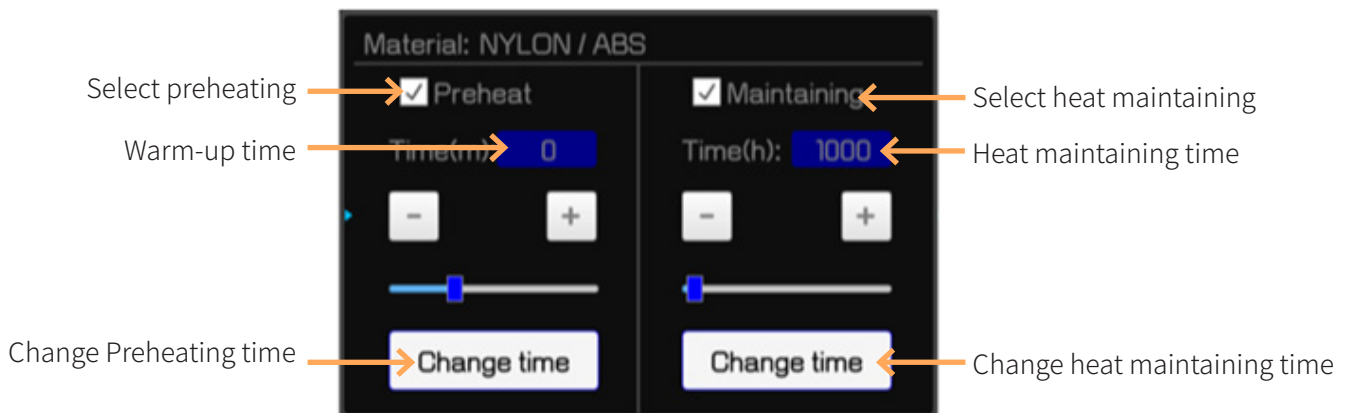
Figure 4. 8 Setting interface for preheating and heat maintaining
