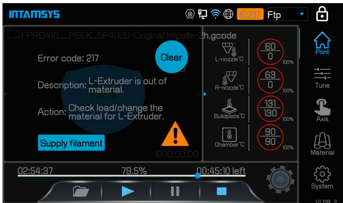
Figure 5. 10 Starved feeding alarm interface
