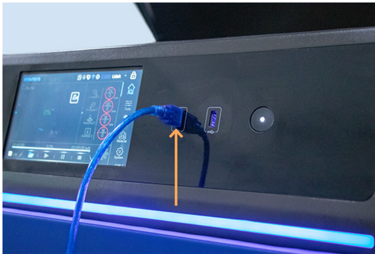
Figure 5. 19 Connection method of USB print mode
